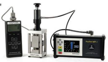
Adhesion testers include everything needed for testing: Adhesion Tester, built-in rechargeable NiMH battery with charger, dollies, abrasive pad, cutting tool, glue with mixing sticks and palettes, cotton swabs, USB cable, PosiSoft Software, instruction booklet and video, shoulder strap (AT-A only), Certificate of Calibration traceable to NIST, two-year warranty, and sturdy, lightweight carrying case
