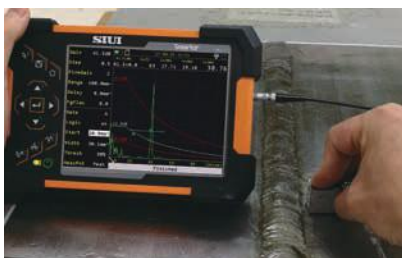
● Flat weld testing
