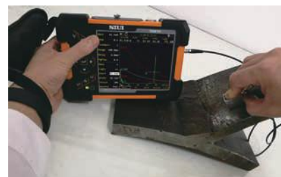
● Angle weld testing
