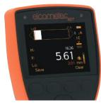
In scan mode the gauge takes readings at a rate of 16 Hz (16 readings per second).
