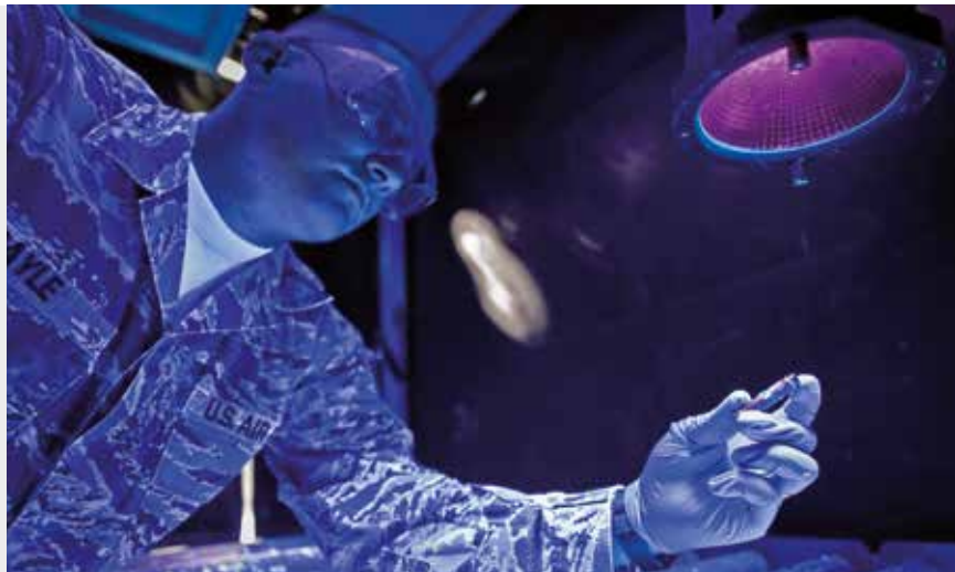
NDI Technician of the 86th Maintenance Squadron takes a closer look at a nose landing gear wheel bolt during a magnetic particle inspection at Ramstein Air Base, Germany.
