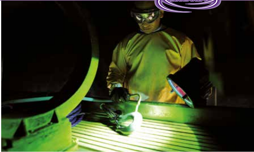
NDI Technician of the 437th Maintenance Squadron checks a cracked chrome panel from a C-17 with a Labino BB 2.0 Series at Joint Base Charleston, S.C.
