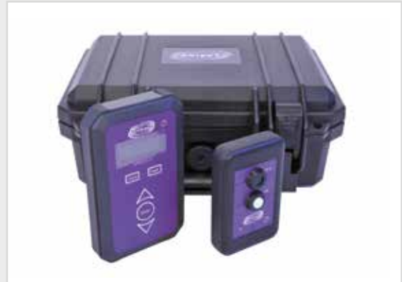
APOLLO 2.0 SINGLE KIT PACKAGE INCLUDES: Reader unit, Sensor unit, Calibration certificate, Carrying case.
