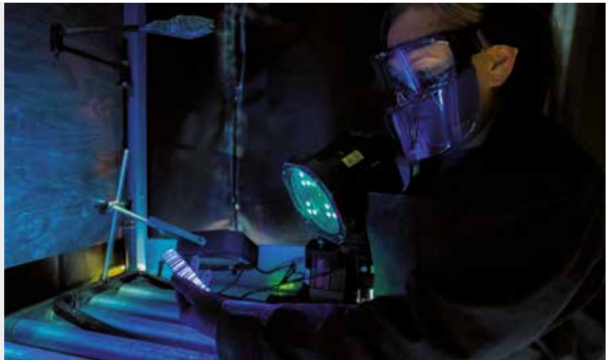
NDI Technician of the 437th Maintenance Squadron checks a cracked chrome panel from a C-17 with a Labino BB 2.0 Series at Joint Base Charleston, S.C.
